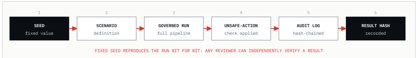
Figure 5. Simulation validation workflow. A fixed seed and a scenario definition drive each run; the governed pipeline executes; an unsafe-action check is applied; the run is written to a hash-chained audit log and a result hash is recorded.
